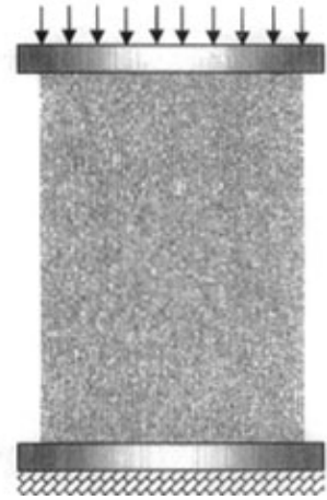
图 2.6 岩石试件仿真加载系统 Fig. 2.6 Simulated loading system of rock specimen
